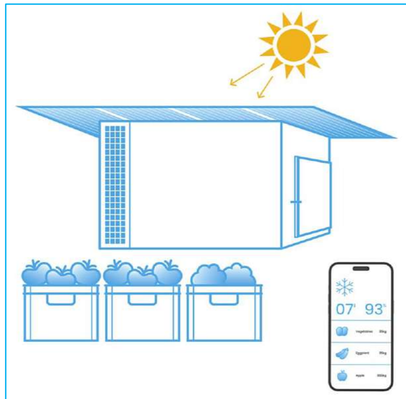
Schematic diagram of Oonnayan Solar Cold Storage and accompanying app for monitoring the produce’s shelf life. The latter was developed by BASE under the Your Virtual Cold Chain Assistant (YVCCA) project .
