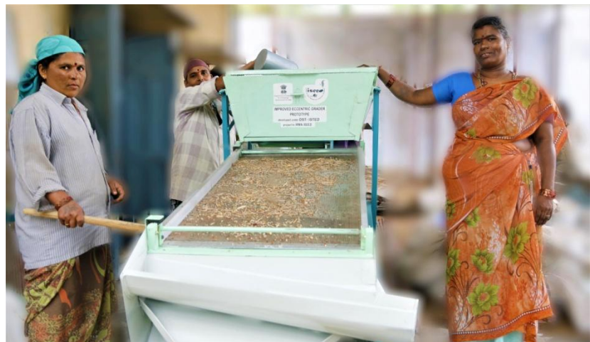
The multi-purpose grader developed by Earth 360 with support from ISEED. The machine has been designed to save power and is operated by women.
